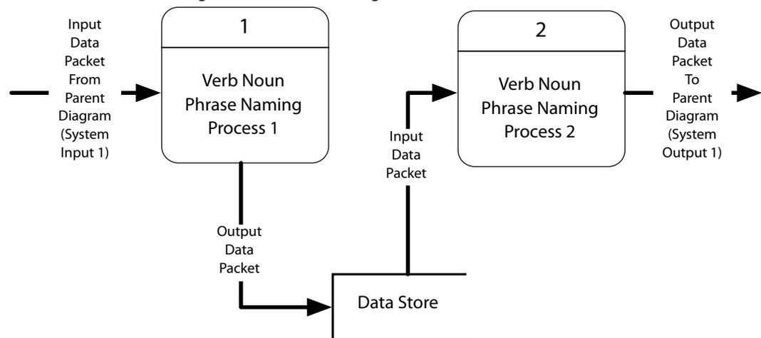
Figure 9–2: Data Flow Diagram (Yourdon Notation)
